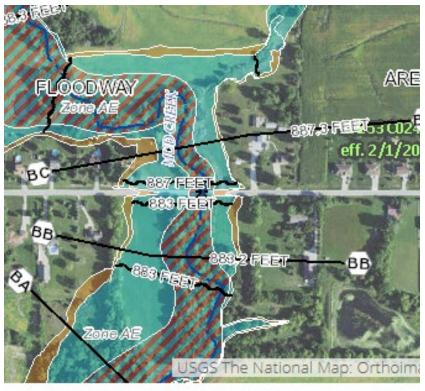
Floodplain portion carrying water flow and where the flood hazard is the greatest:
