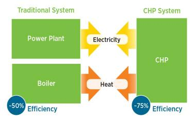
**Figure 1: Diagram of CHP Operations**
